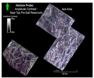
**Figure 4** - 3D seismic attribute showing structural discontinuities in red (rift faults). Variation in the structural trend is observed between the Jupiter and Iara areas, changing from NE-SW to N-S.
