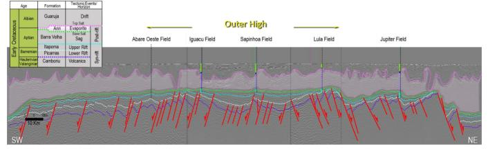
Figure 6 - 3D seismic composite section in depth through some of the major pre-salt oil discoveries in Santos Basin.
