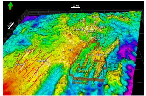
*Figure 7 - 3D* structural view in depth of the near top of the pre-salt reservoirs showing the major oil discoveries (white polygons) in the Santos Basin. Exploration opportunities are indicated by yellow polygons.
