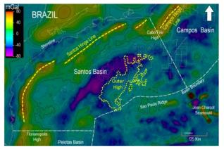
**Figure 1** – Free-air gravity anomaly map of the Southeastern Brazilian Margin (Sandwell et al., 2014). Yellow dashed and dotted lines are the major structural features; i.e., basin hinge lines and Outer High. Thin white dashed polygons indicate awarded blocks.
