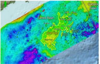
**Figure 2** - Depth structural map of the base salt or near top of pre-salt reservoirs in the Santos Basin. Outer High, the major structural feature in the basin, is highlighted in yellow.
